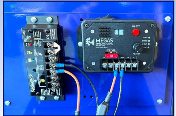
*Streamlined controls inside battery box*
